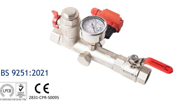
Applications Engineering Dual port fire sprinkler valve set has been specifically designed for the residential & Domestic market, using our own flow switch that has been specifically designed for the valve set to activate at 25 l/min. A monitored Ball valve can be retro fitted and using our unique design also gives the option to monitor to the flow switch
