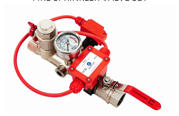
Applications Engineering Dual port monitored fire sprinkler valve set has been specifically designed for the residential & Domestic market, using our own flow switch that has been specifically designed for the valve set to activate at 25 l/min. The monitored Ball valve can be retro fitted and using our unique design also gives the option to monitor to the flow switch
