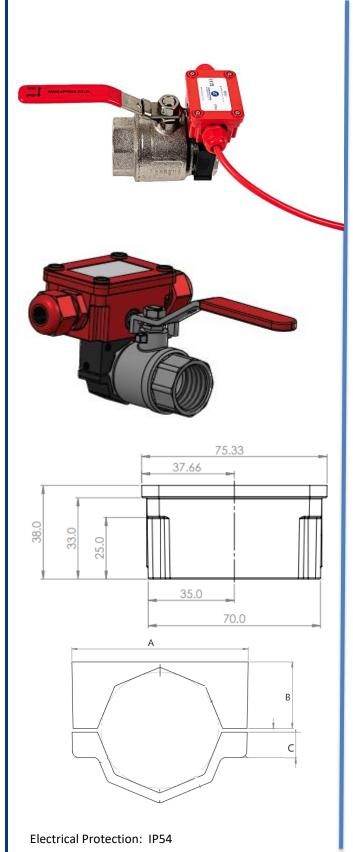
Applications Engineering's Monitored Ball Valve (MBV) is designed to monitor the fully open position of a ball valve. The MBV has a toggle switch, which is activated when the ball valve handle is moved from the fully open position.
