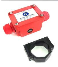
The MBV is a 3-piece construction that makes mounting easy and fully retrofittable to any Applications engineering Ball Valve or valve set. The 2-piece clamp is secured around the fixed hex position of our ball valve using locating lugs and the housing can be easily screwed into place from the top of the clamp with nuts pre-moulded into the lower clamp.
