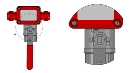
After wiring as required secure the lid to the MBV housing with the remaining four screws supplied.
