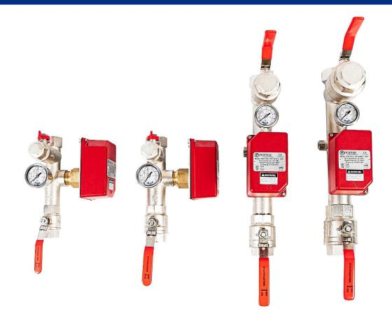
Applications Engineering Dual port fire sprinkler valve set has been specifically designed for the residential & Domestic market using a Potter VSR-S series flow switch. A monitored Ball valve can be retro fitted and using our unique design also gives the option to monitor to the flow switch
