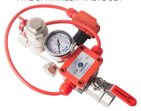
Applications Engineering Dual port monitored fire sprinkler valve set has been specifically designed for the residential & Domestic market, using our own flow switch that has been specifically designed for the valve set to activate at 25 l/min. The monitored Ball valve can be retro fitted and using our unique design also gives the option to monitor to the flow switch
