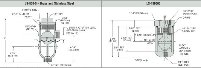
+L<sub>1</sub>= Switch actuation level, nominal (based on a liquid specific gravity of 1.0).
